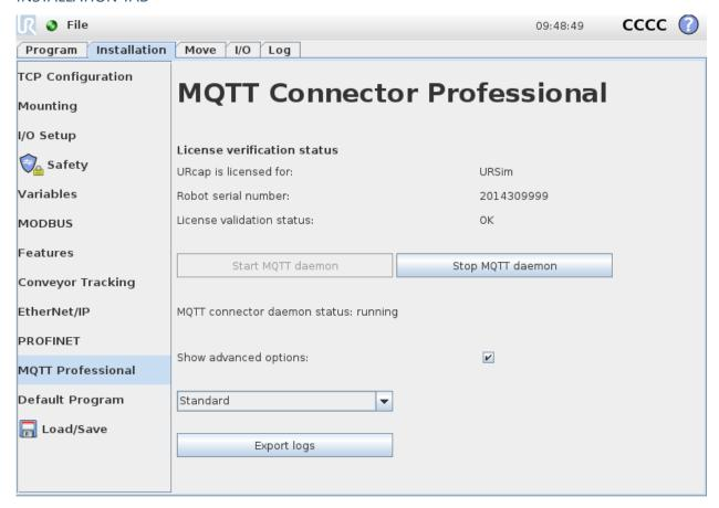
Installation tab incorporates buttons to start and stop MQTT daemon. Also licensing details are displayed. Since URCap version 1.3.0, all simulator versions use one common license, indicated by URSim designation in serial number label. Physical robots require purpose built URCap with correct serial number.
