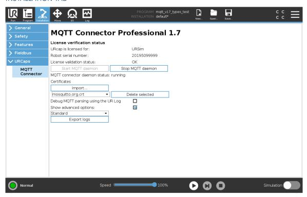
Installation tab incorporates buttons to start and stop MQTT daemon. Also licensing details are displayed. Physical robots require purpose built URCap with correct serial number.
